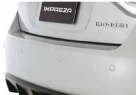
Rear parking sensors
